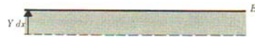
Fig. 3-8-1 The shaded area indicates the energy range occupied by states with a value of \partial E_r / \partial x = Y , whose energy changes from a value smaller than E to one greater than E when the external parameter is changed from x to x + dx .
