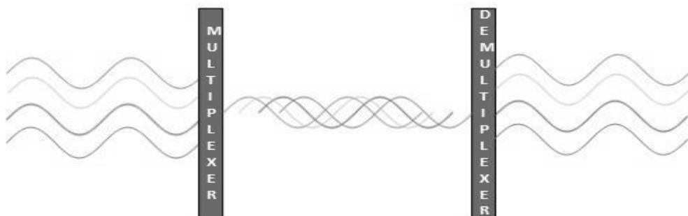
Wavelength Division Multiplexing
